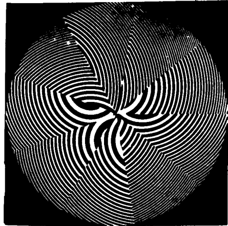
Fig. 3. Amplitude mask of a focusator concentrating the irradiance of a CO 2 laser into a pattern of dots (left).
